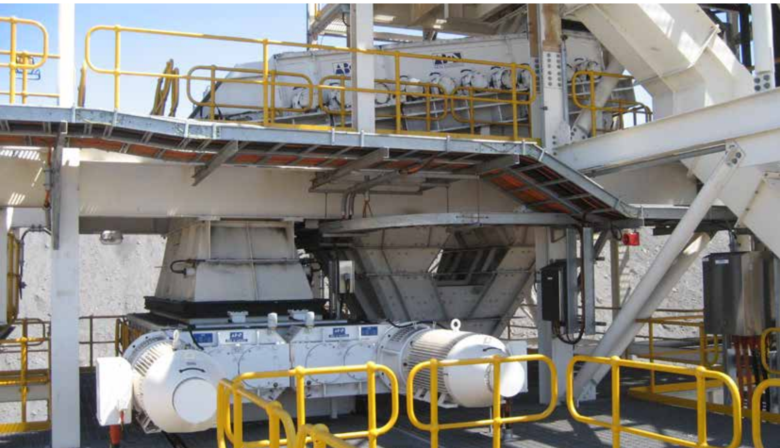
▲ ABON Rollerscreen installed over an ABON Tertiary Sizer
