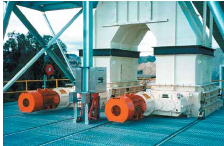
Tertiary Sizers via Bifurcated chute ▲
