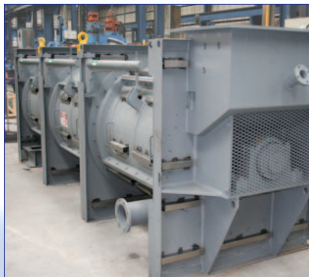
A modular AST Dryer ready to be fitted with thermal insulation in the Atritor workshop.
