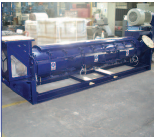
An AST Dryer for drying mica ready to be shipped to Finland.
