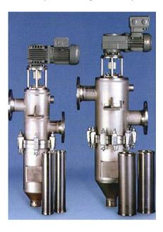
The liquid flows from the outside to the inside of the wedge wire screen and leaves the filter housing through the higher placed exit. Between the lower placed entrance and the upper exit a seal is placed, limiting any cross contamination between lower (dirt) part and upper (clean) part.
