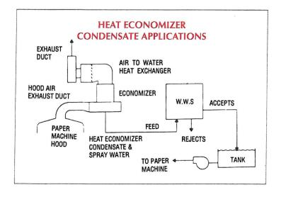
Concentration and spray water is bleed from the economizer circuit to recover fibre being airborn from the dryer. The normally 165 TBC will recover the fiber for return to make-up. Fines and dust will pass through the screen.
