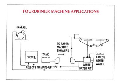
These should be the most common type of applications with the WWS being installed as "insurance" against material getting to the showers and other end uses that could cause operating problems. We have shown a Disc type save-all in the flow diagrams, but the flow set-up would be basically the same regardless of the type. The filtered water from the WWS would be ready for shower water use with no further filtration required.
