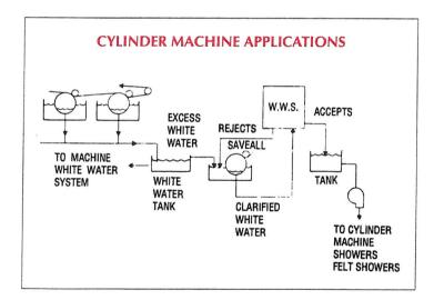
The mesh required is typically 105 micron opening and depending on the concentration of fiber, 150 mesh M. G. or the 165 TBC would be used. The market grade (M. G.) screen is stronger and can accept higher fiber concentration.
