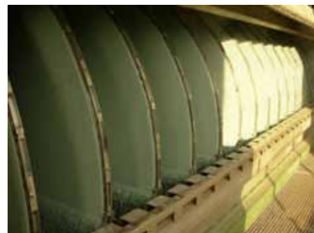
8-disc Lime Mud ClariDisc® operating at a Pulp Mill in Portugal.
