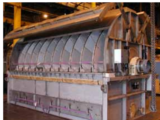
10-disc Lime Mud ClariDisc® ready for shipment to a Canadian Pulp Mill.
