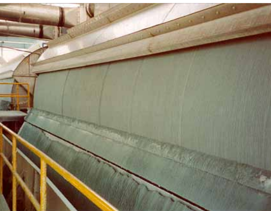
2-118 m 2 EIMCO® Lime Mud Precoat Filters operating at an Indonesian Pulp Mill.
