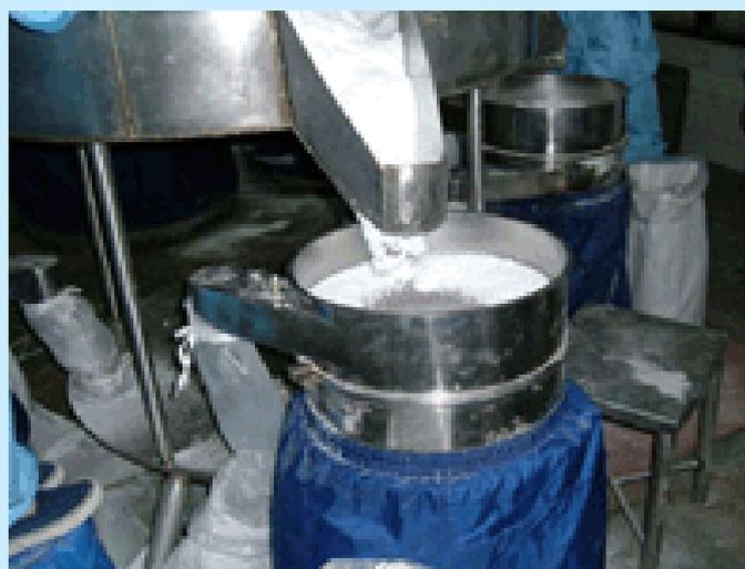
From a chemical factory. Their target is to dewater from the granules. They choose MCL-800-1 with 100 mesh sieve. The reference capacity is 300 kg/h. The contact part is stainless steel 304(GMP standard). The mesh material is Stainless steel 304.
