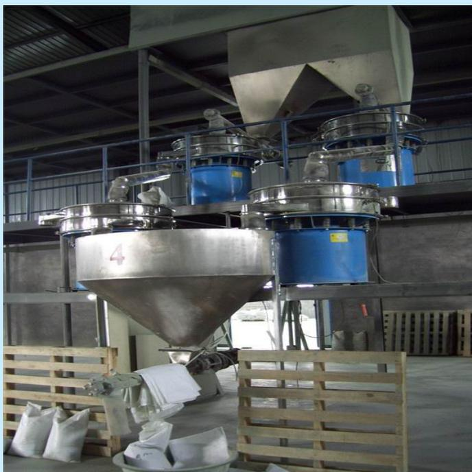
From a spices factory. They choose the MCL-1500-1 with 30# and 20# (mesh size). The reference capacity is 3t/h. The contact part is stainless steel 304(GMP standard). The mesh material is Stainless steel 304.
