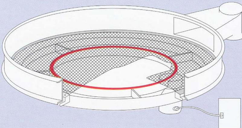
Sonoscreen can be installed or retrofitted in any operational vibrating screen. Items needed are an ultrasonic generator, ultrasonic screen resonator with transducer and high frequency cable connector.
