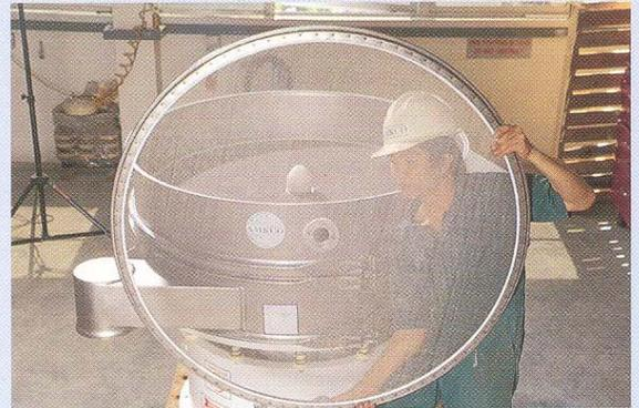
**MINIMUM SCREEN BLINDING** for all separation processes is achieved through the use of and the combination of several techniques. The vibration of the Separator, the use of sliders, the use of bouncing balls, the use of ultra-sonics, the use of water sprays, the use of wipers, and last but not least, the use of good well tensioned screens.
