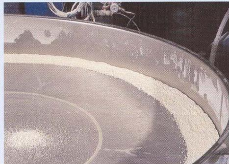
**NEW FOOD PRODUCT** made possible with ultrasonic application to the screen. The material would not process at the required screen mesh. Now, the end product is unique with fast pay back to the producer.
