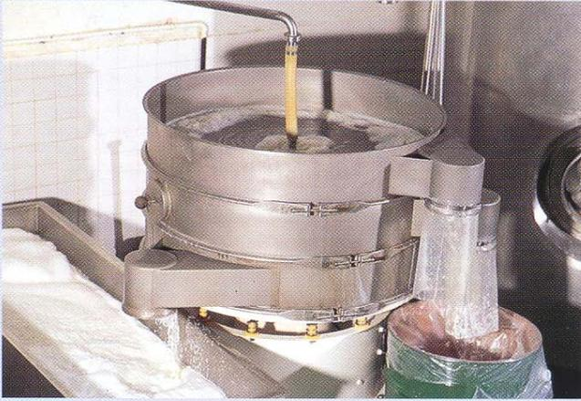
**NO TRANSMITTED VIBRATION** was a need for a dairy and juice producer. The AMKCO is mounted on a portable stand, easily moveable to different locations for different products. The various locations have floors that are not always level. Quick and easy shims under the legs keep the screen level for good separation.
