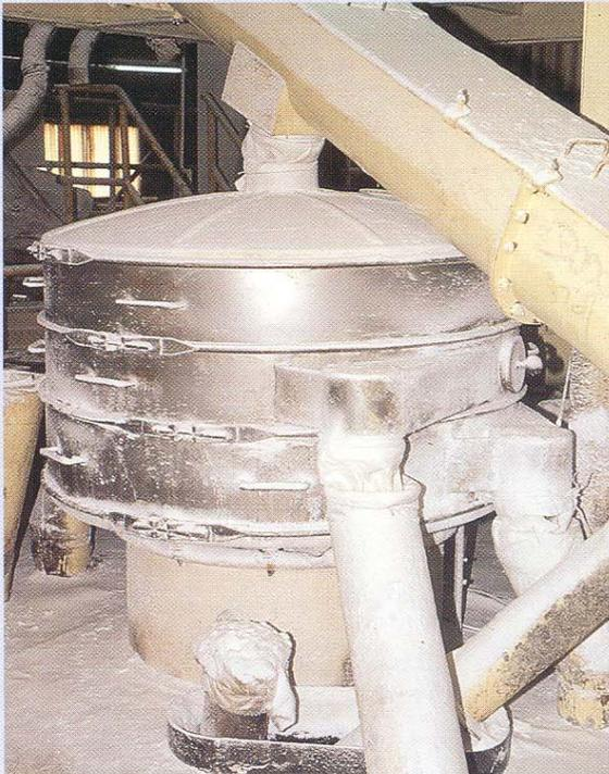
**QUICK AND EASY SCREEN CHANGE** are obtained by a sugar producer using a 2-deck Separator to simultaneously classify sugar into 3 products. The users market has several different specifications requiring fast and easy screen changes. For smaller units, quick release clamps and no screen center tie downs make changes even faster.
