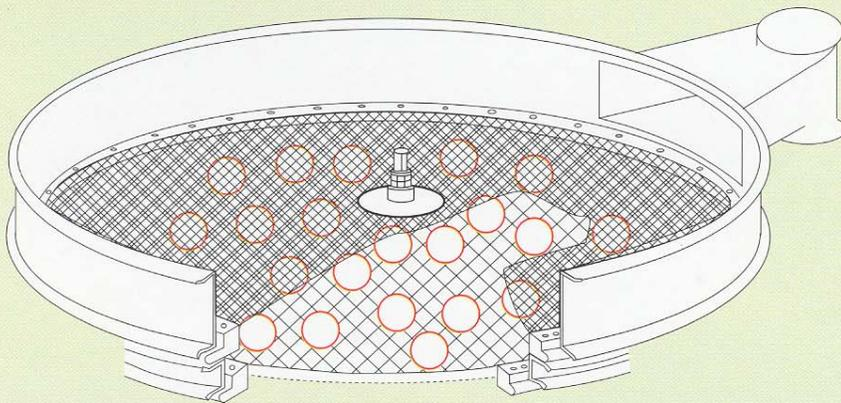
These bouncing balls are available in natural rubber, neoprene, silicone, EPDM, polyurethane and nitrile. Sizes range from 16, 22, 25, 28, 35 and 50 mm in diameter.
