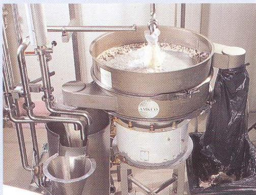
**LONG SCREEN LIFE** is our goal. Removing fiber from coconut milk prior to packaging adds little to the cost of the product because the screen lasts nearly a year. Proper tension, high quality wire, and bonding or welding achieves quality product at low cost.
