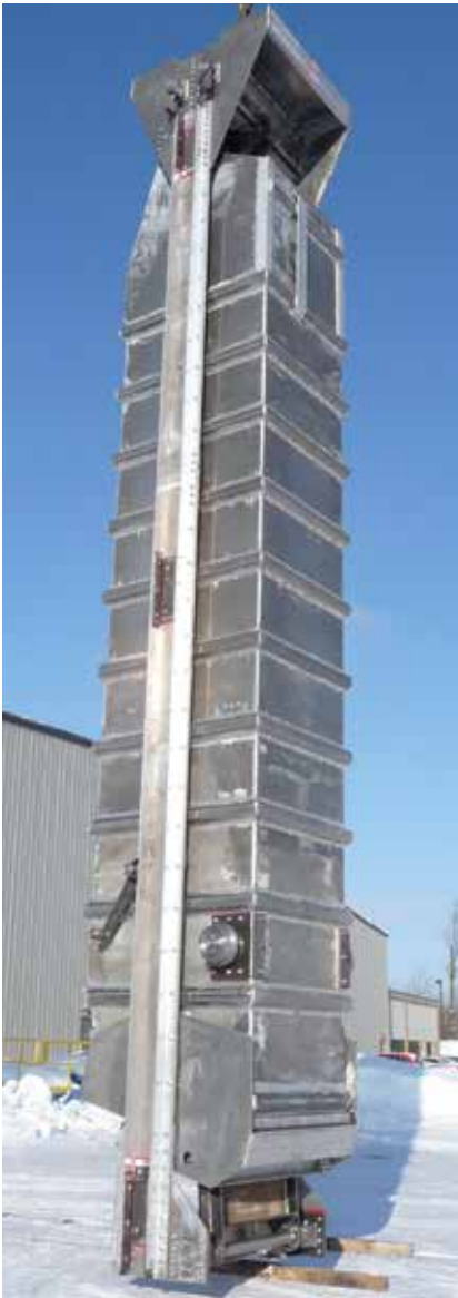
The standard Dorr-Oliver Aluminum Bottom Dump skip is the workhorse of the hardrock mining industry. ▲
