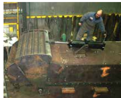
These photographs show a Measuring Flask with an ARC GATE door discharge chute that is particularly well suited in limited space and where very accurate flow control is required.
