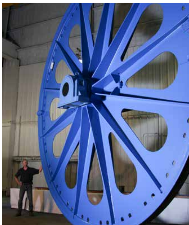
Largest Sheave in North America 21.5 ft ~ 6.6 m diameter
