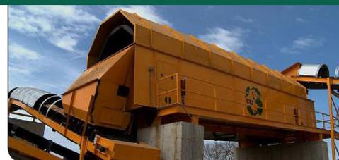
Trommel Screens effectively separate out fines from over-sized material. Ideal for applications requiring final product to be 2-inch and smaller.
