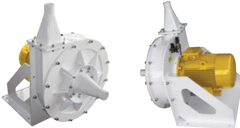
These machines are designed specifically for killing insects, eggs or larvae present in the flour by a violent impact of the machine. They extends the storage of the materials for longer periods. They are operated by a motor directly drives the rotor.
