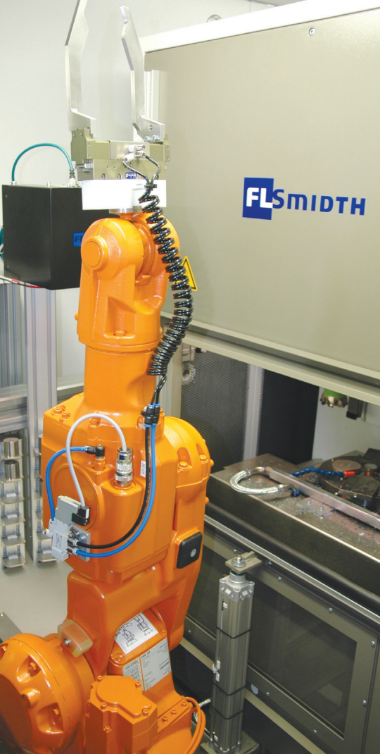
PAL-MIL_R operated by industrial robot in a Nucleus-C system
