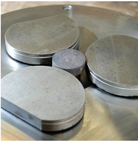
Dedicated clamping device for round samples
