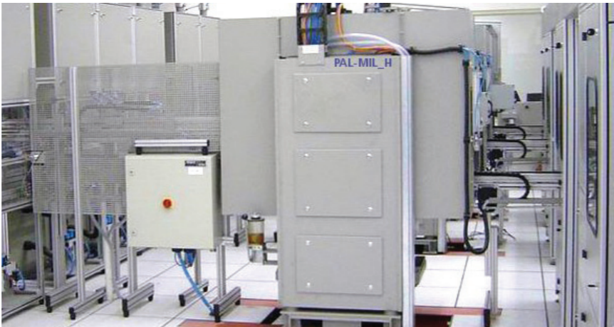
PAL-MIL_H integrated in a linear sample processing system
