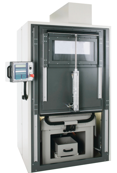
Integrated easily accessible box for collecting milling cuts
