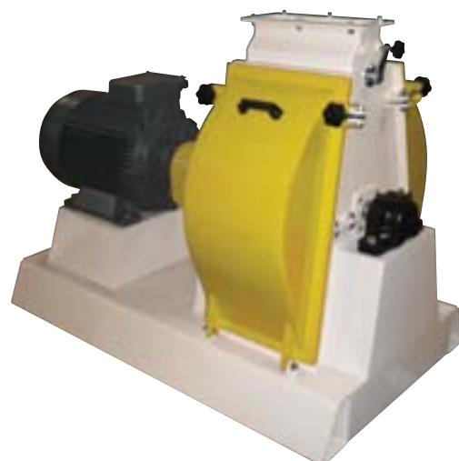
Hammer mills are used to grind screening, grain husk etc. The material is fed by a feeder. The grinding process is made between moving blades and perforated sleeve. The rotor consists of a steel shaft, hammers on the shaft. Rotor shaft is heat treated and felt holes are sand blasted. Hammers are strengthened abrasion proof with heat treatment. Doors for replacement for sieves designed for easy and fast replacement and maintenance.
