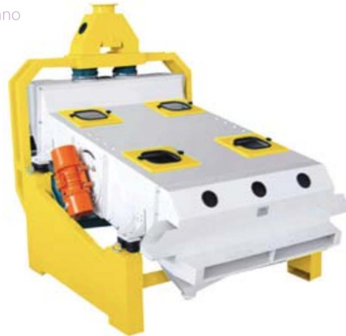
The grain separators are used to separate the coarse and fine impurities from cereal both for precleaning purposes for cereal storage systems and for main cleaning in flour mills for effective cleaning. The principle of the separation is based on the kernel size.
