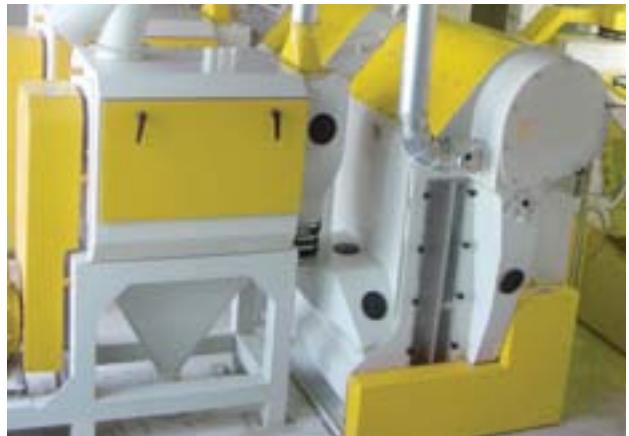
The radial tarars are used to separate dust, light purites, broken kernels and etc. from a grain. The system has an advantage to reuse most of the air without exhausting and without requirement of central or special filter and aspiration system which lowers energy consumption.
