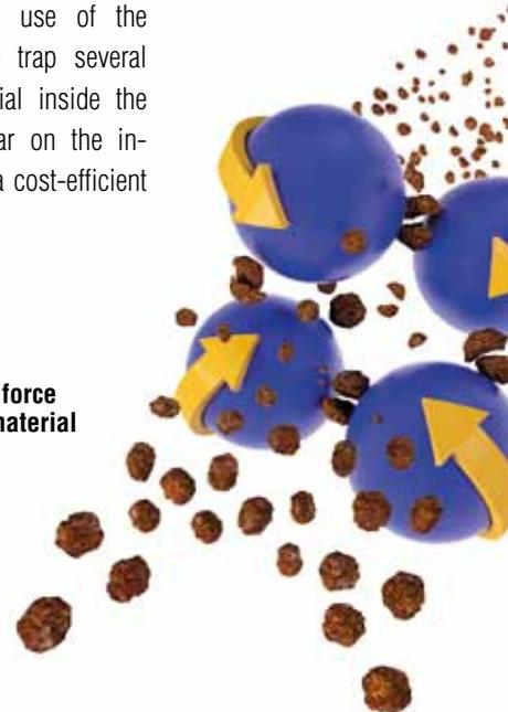
during operation protective layers of grinding balls fill and remain inside the grid segments
